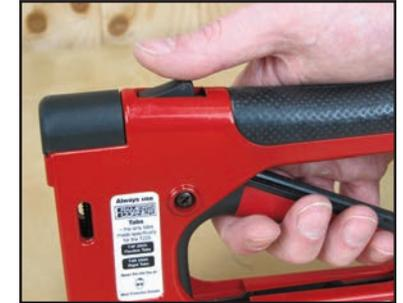
Pull the magazine cover up to reveal the loading slot
