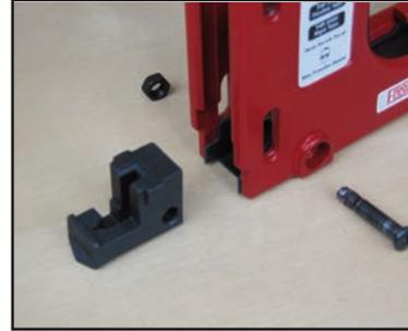
When new, the tab drive is lubricated. Over time it may be necessary to reapply lubrication. It is not recommended you undo all the screws holding the driver together as there are several springs contained inside, and they are difficult to reassemble.
