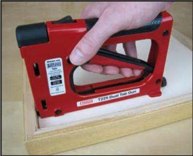
2) Ensure the frame is held securely so it will not move as the tab is inserted.
