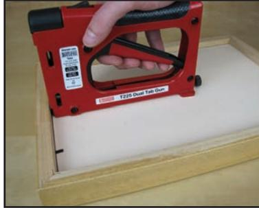
6) For frames up to 300mm x 300mm we recommend using 2 tabs on each side ( Total 8 ). Larger frames may require more tabs.
