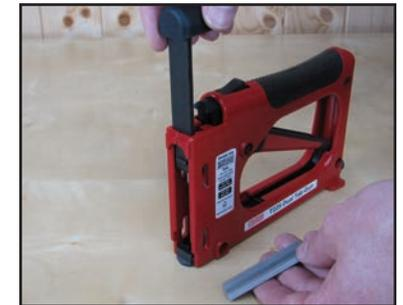
Load a strip of T4F or T4R tabs into the magazine with pointed end forwards
